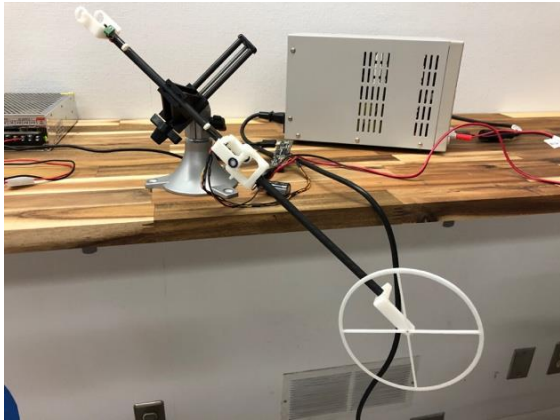
Figure 10: Robotic arm device controlled by a NiTi wire actuator
